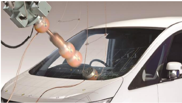
Figure 9. Impact test for assumption of pedestrian head, [14]
