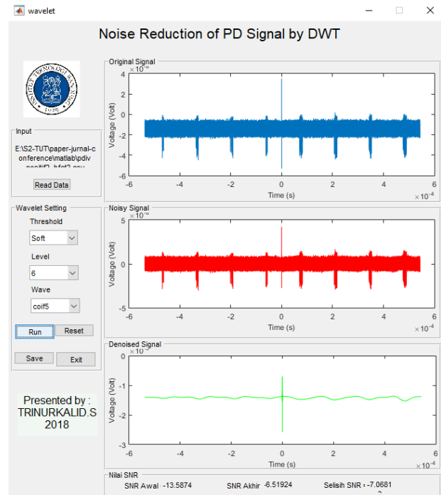
Figure 13. HFCT Denoising Signal Soft Threshold, level 6, coif5 wavelet type
