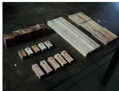
Figure 3. Bakau timber testing sample
