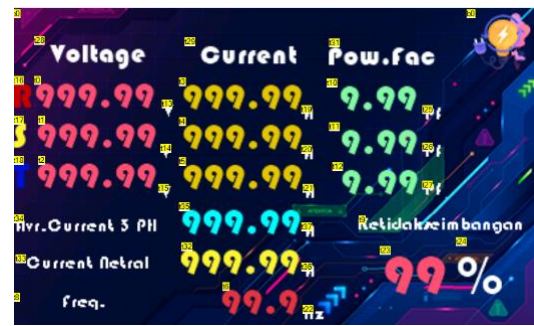
Figure 5. Human Machine Interface (HMI) design on the Nextion LCD
