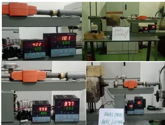
Figure 10. Tensile load furnace
