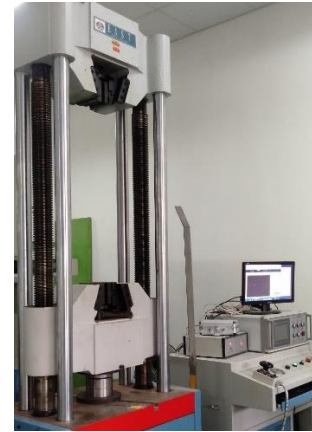
Figure 2. 200 Mpa compaction process using Universal Testing Machine
