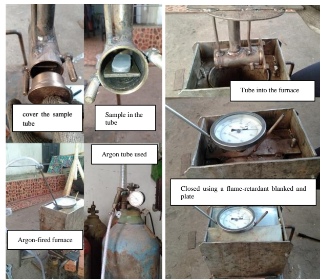
Figure 3. The sintering process takes 3 hours with a temperature of 500°C, and the furnace is supplied with argon gas
