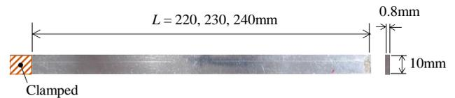
Figure 1. Geometry of an aluminum cantilever beam
