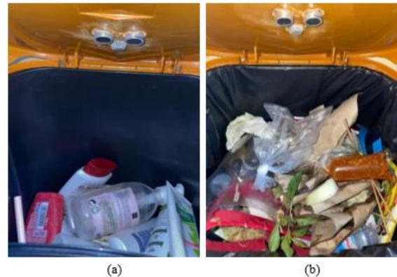
Figure 7. Testing the MQ-4 sensor in a trash can with (a) inorganic trash and (b) organic trash
