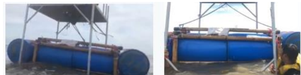
Figure 2. H-Beam type wave energy converter (WEC)
