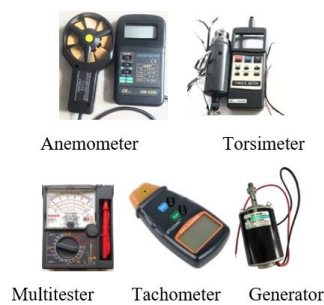
Figure 6. An apparatus consists of a digital anemometer, tachometer, digital torque, multimeter, and a generator
