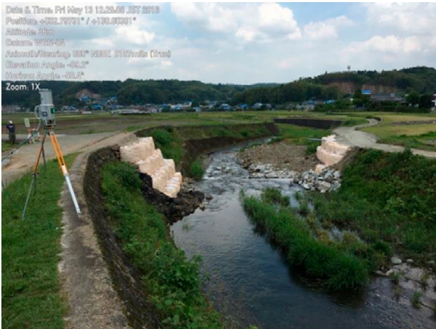
Fig. 7. The terrestrial LiDAR setup and damage to the canal embankments. The main fault crossing is at the location of the repairs visible in the photograph.
